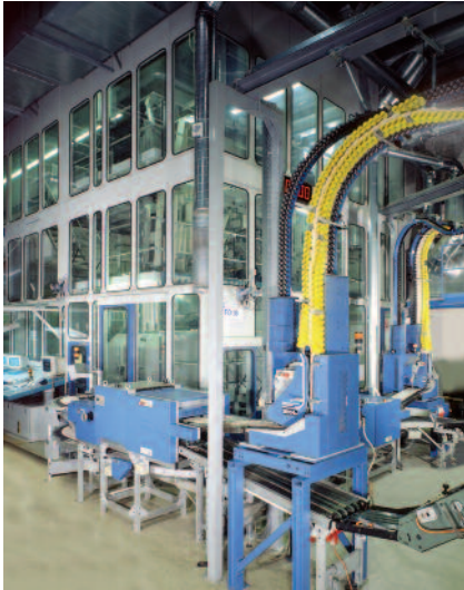
The overhead transport system Newsveyor can handle up to three shingle streams together to transport a larger number of copies per running metre and thus has lower costs than single-gripper systems.
