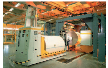
Intermediate transport systems will need a larger capacity to handle increased weight but fewer units may be needed to handle 31% fewer rolls.
