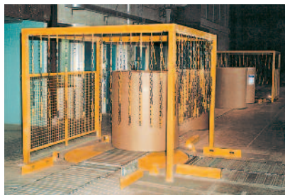
Conveyors will need to be able to handle increased roll weight and width, whilst turns require more space.
