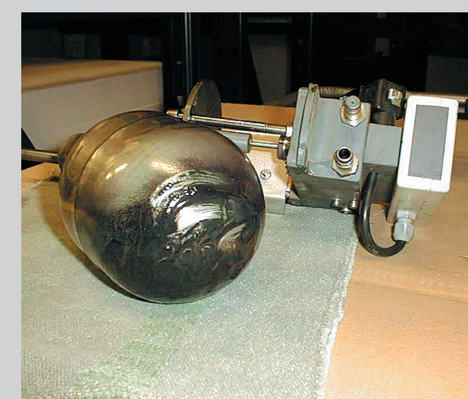
Dirt build-up on the alcohol stabiliser float adds to its weight and can change the alcohol content in the dampening solution. Photo Technotrans.
