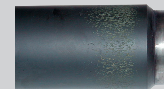
Roller damaged due to uneven setting that has significantly increased running temperature. Photo Böttcher.
