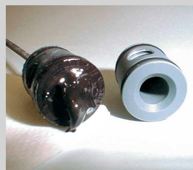
An inline ejector nozzle contaminated with ink from either using the wrong filter element or poor maintenance. Photo Technotrans.
